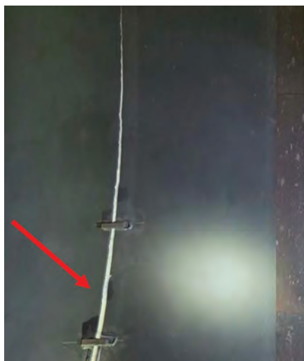
IAFD. Flow shield and EJ frame cracking caused by thermal growth and stress concentration at the flange base, leading to repeat weld repairs
