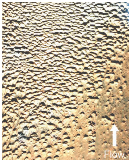
3. Single-phase FAC example (left) at HP economizer inlet showing chevron/horse-shoe attack in the flow direction. Shallow, dark "dimple" morphology indicates two-phase FAC attack in LP evaporator tubing (right)
