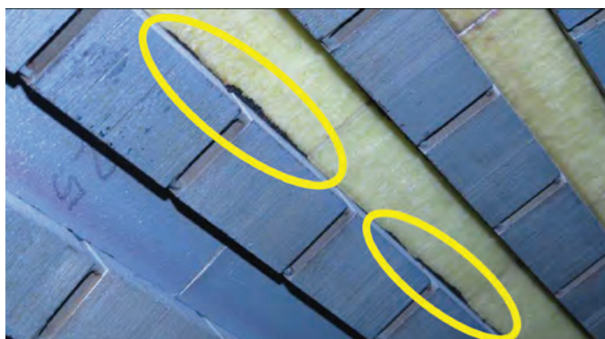
Grease tracking at stator slot wedge interfaces (left) and at end-winding support blocks (right), indicating relative movement and vibration that warrant wedging and support checks
