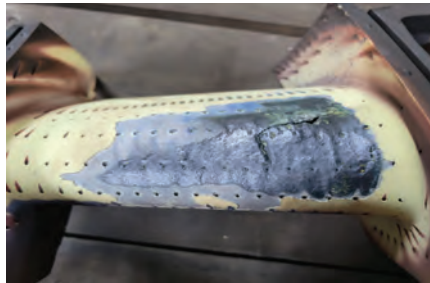
Thermal barrier coating spallation traced to iron contamination, leading to coating failure, base metal exposure, and vane degradation
