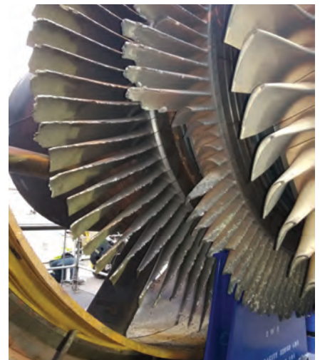
R3 blades exhibited creep damage and liberation, traced to elevated temperatures during low-load operation
