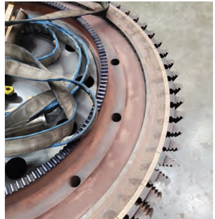
Threading and machining restored proper air separator fit after fretting damage, ensuring correct compression and long-term rotor integrity
