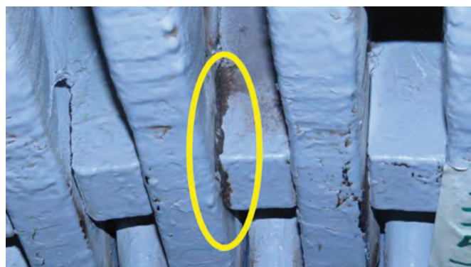
Grease tracking at stator slot wedge interfaces (left) and at end-winding support blocks (right), indicating relative movement and vibration that warrant wedging and support checks
