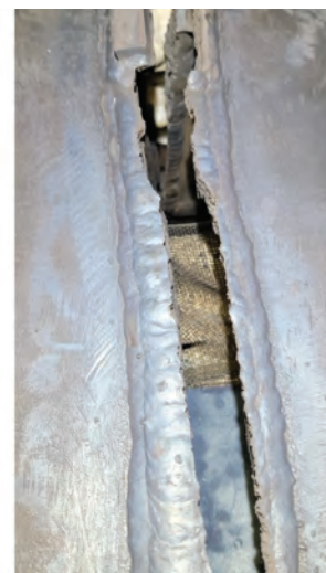
IAFD. Flow shield and EJ frame cracking caused by thermal growth and stress concentration at the flange base, leading to repeat weld repairs
