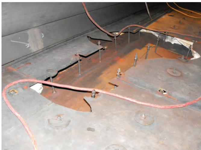
HRST. Square duct liner failure from thermal fatigue and distortion 9 (left). Threaded stud failure caused by vibration and inadequate weld integrity (right)
