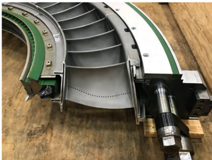
TRS Services. Shop assembly allows TBR roundness and flatness verification, precise vane and seal installation, and delivery of outage-ready assemblies
