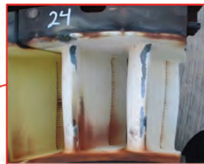
Entrust Solutions. R2 vane TBC spallation and oxidation attributed to coating durability and cooling design deficiencies, consistent with fleetwide design issues
