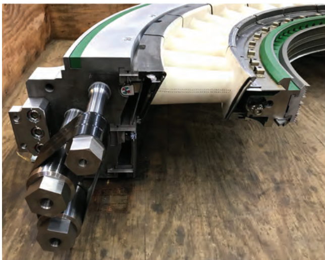
TRS Services. Shop assembly allows TBR roundness and flatness verification, precise vane and seal installation, and delivery of outage-ready assemblies
