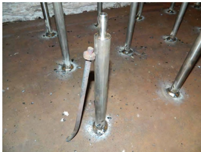
HRST. Square duct liner failure from thermal fatigue and distortion 9 (left). Threaded stud failure caused by vibration and inadequate weld integrity (right)
