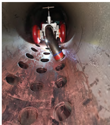
3. Internal access tool deployed in header, modular carriage aligned to push RFET probes up individual tubes
