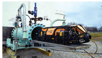
1. Crawler inspects storage tanks in-service, using PAUT to map corrosion while eliminating confined-space entry and downtime
