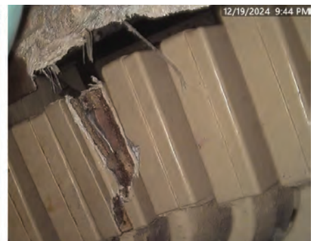
2. Components damaged by a liberated generator cooling fan blade include the gas shield and stator end cap. Root cause was one bolt breaking, caused by overtorqueing, and a second bolt breaking from fatigue failure
