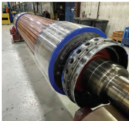
7. Alstom generator field
