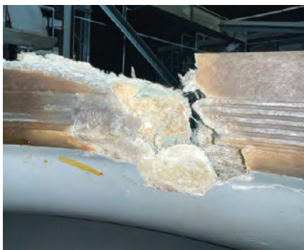
2. Components damaged by a liberated generator cooling fan blade include the gas shield and stator end cap. Root cause was one bolt breaking, caused by overtorqueing, and a second bolt breaking from fatigue failure
