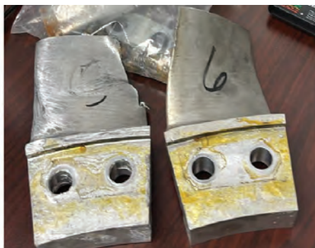
2. Components damaged by a liberated generator cooling fan blade include the gas shield and stator end cap. Root cause was one bolt breaking, caused by overtorqueing, and a second bolt breaking from fatigue failure
