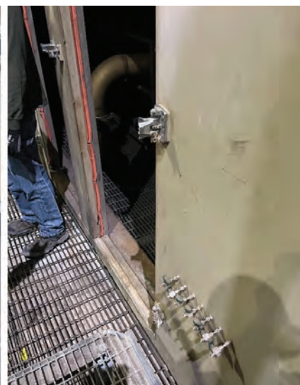
7. Combustion can hardware was damaged after one can “violently disassembled,” strong enough to blow off the compartment door
