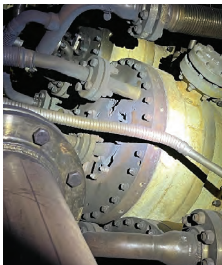
7. Combustion can hardware was damaged after one can “violently disassembled,” strong enough to blow off the compartment door
