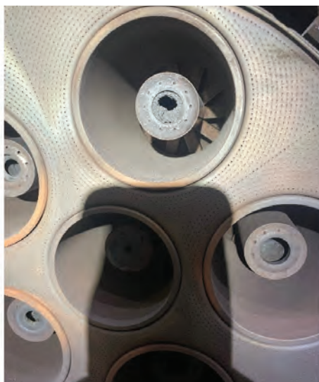
7. Combustion can hardware was damaged after one can “violently disassembled,” strong enough to blow off the compartment door
