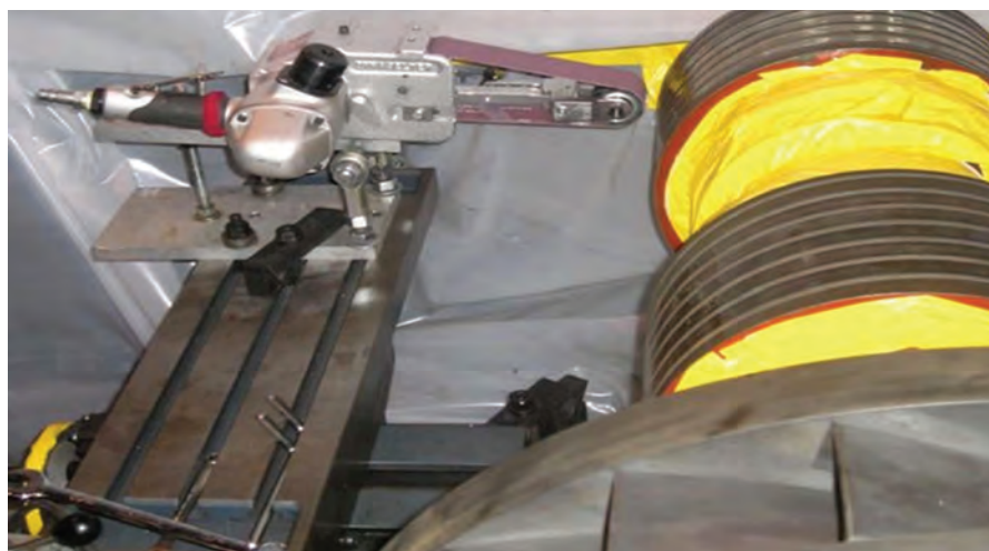
15. Machine can resurface two collector rings on-site typically in two shifts while the field is on turning gear, removes around 0.01 in. of metal
