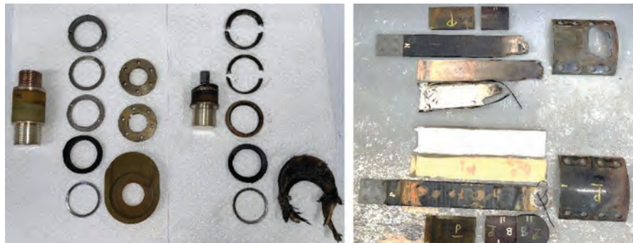
13. Side by side comparison of damaged vs undamaged radial (left) and axial (right) leads. Damage was discovered after ST trip on high vibration in bearing No. 6 and exciter bearing
