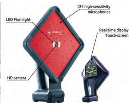
5. Methane leak detection in GT fuel distribution piping is just one of several applications (air, H2) for hand-held acoustic detection method based on pictured sensor operating up to 25 feet away
