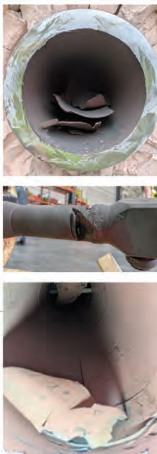
3. Liberated HP attemperator liner pieces were discovered in the downstream piping, resulting in replacement of nozzle, steam/lance, and 80% of P91 piping, along with significant weld repairs
