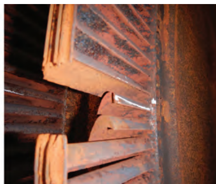
9. Example of damage to blade rows 1-4 of the LP steam turbine discovered during a 2025 inspection. EPRI guidelines were followed for rotor weld repair
