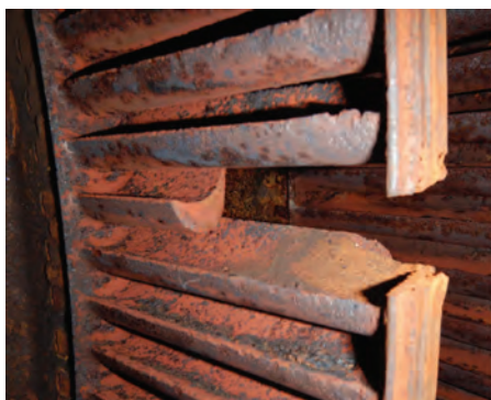
9. Example of damage to blade rows 1-4 of the LP steam turbine discovered during a 2025 inspection. EPRI guidelines were followed for rotor weld repair
